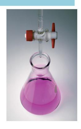
In this titration, HCl, analyte, is in the Erlenmeyer flask and NaOH, titrant, is in the burette. Phenolphthalein, which is clear in the presents of an acid and pink in the presents of a base, is added to the HCl. NaOH is added to the HCl and Phenolphthalein until the solution turns pink, which signifies the equivalence point has been reached
